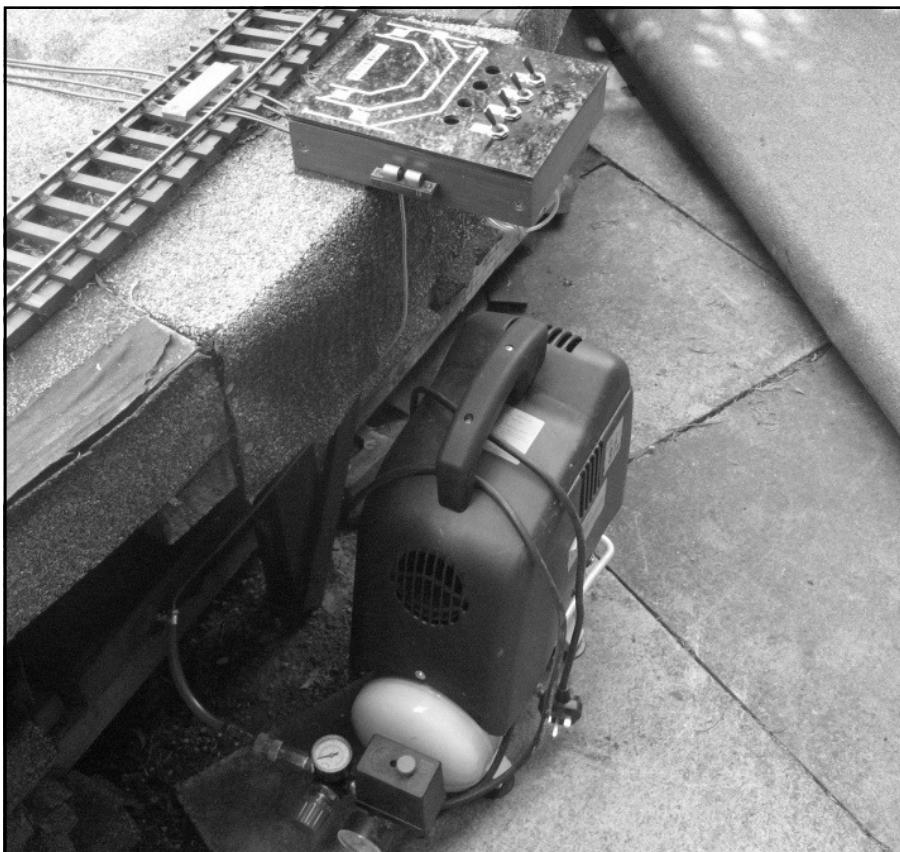
The air supply comes from a portable compressor which is about the size of a toolbox so can be easily carried; the system operates at 40psi and has a temporary electricity supply at the moment. The panel is hinged and can be opened to work on the pipe work as shown in the middle-left picture.
