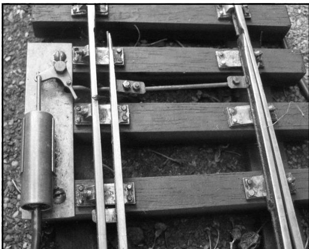
Four "Delair" cylinders and air switches were bought from Brandbright at the A G M, these were built into four turnouts and placed in the garden on the baseboard a year or so before they were connected to an air supply. When I came to operate them I found they jammed on the return stroke. The cylinders are air powered on the outward stroke with spring return.
